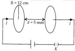
(a) Capacitance of the parallel plate capacitor
