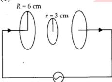
To find magnetic field B of a point 3 cm from the axis within plates, let us assume a loop of radius 3 cm with center on axis. Now modified Ampere's Law.
